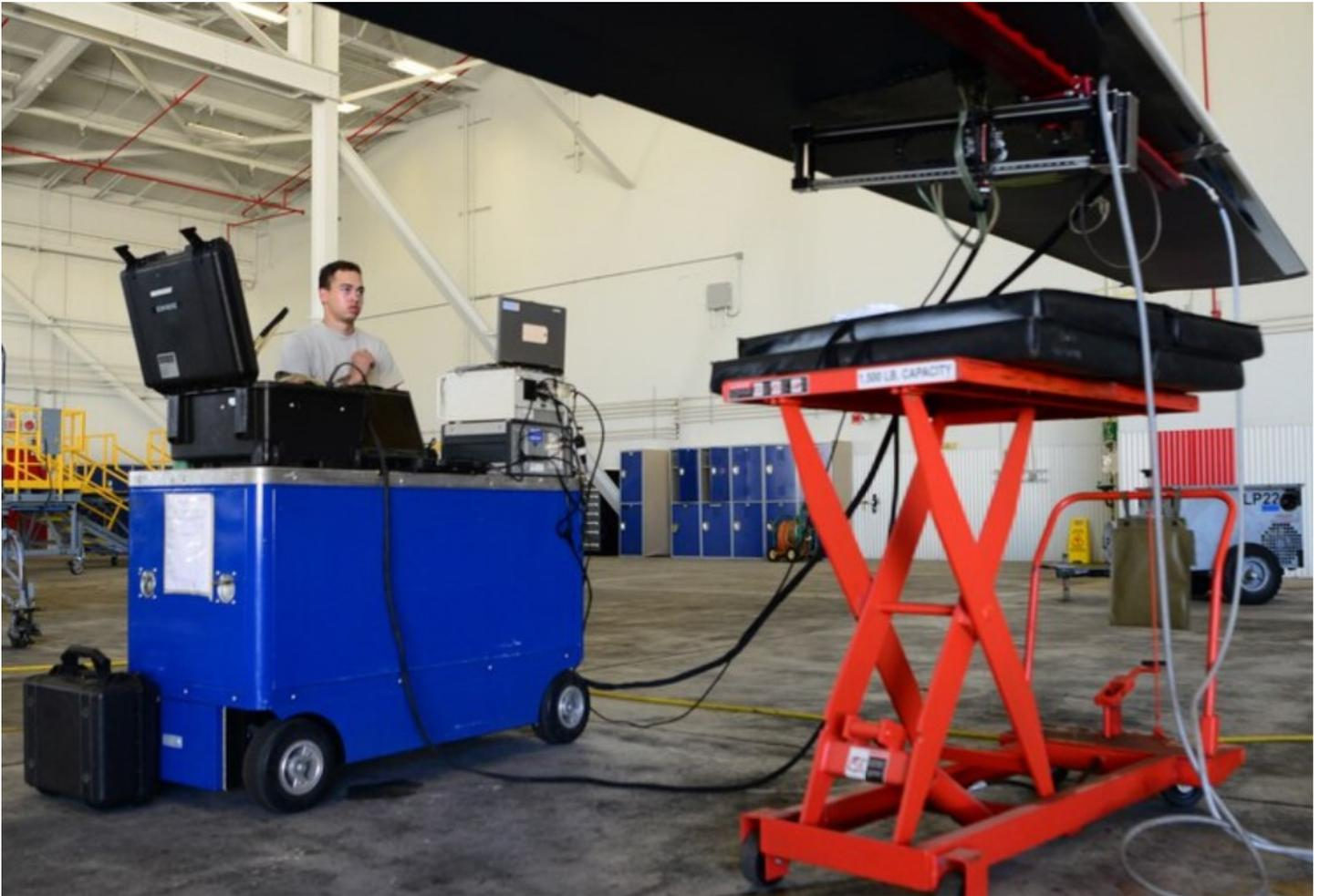
The aluminum alloy cart is customized to store your inspection equipment in one secure place. The portability of the cart provides the flexibility to be moved from one job site to another, while the reinforced top allows it to be used as a workbench in a lab type environment.
