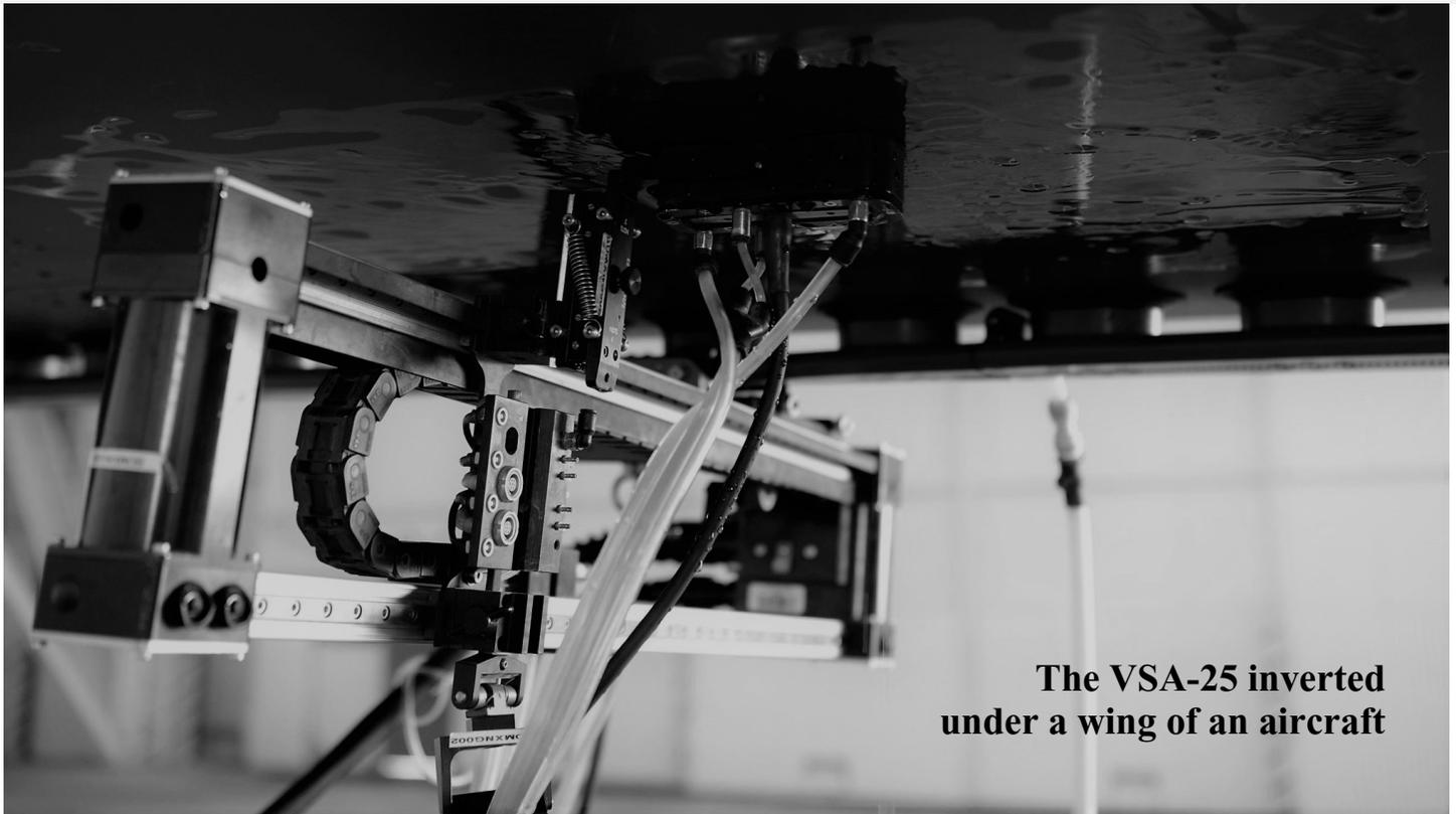
**The VSA-25 inverted under a wing of an aircraft**
