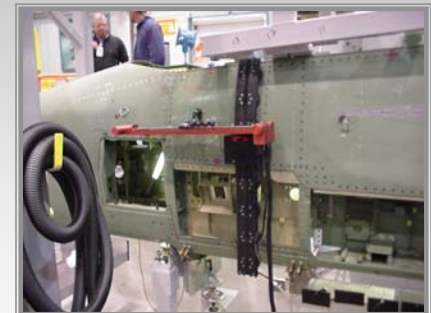
Flexible Track Scanner Positioned on Aircraft Fuselage
