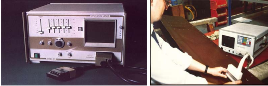
Figure 1. Two generations of NDT array imagers for CFC. Diagnostic Sonar's System 185 (1978) and FlawImager (1988).
